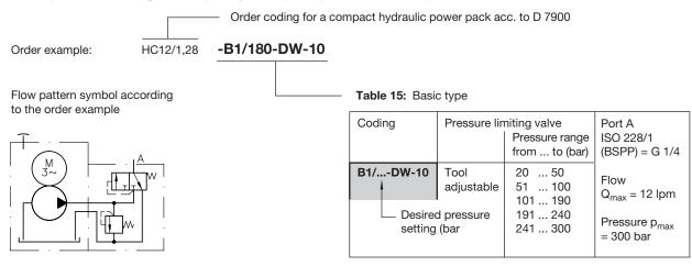
Note: The pressure rating  $p_{max}$  of the compact power pack has to be reduced by 20 bar.
