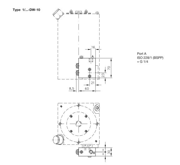
4.5 Version for pipe connection acc. to sect. 2.5
